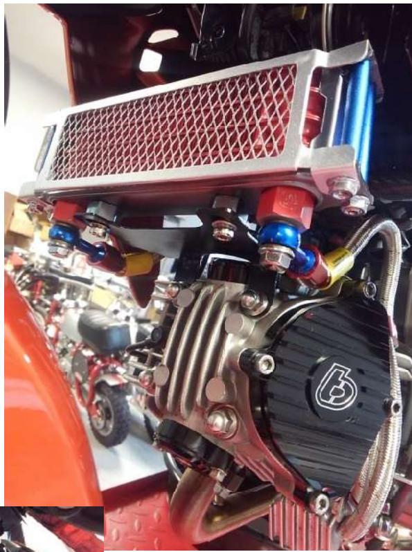
Note- will work with the stock air box but you will have to make a spacer and get a longer bolt to bolt the horn back to its original spot and you will have to bend the main bracket down to make the oil cooler move down and forward away from the air box a little.
