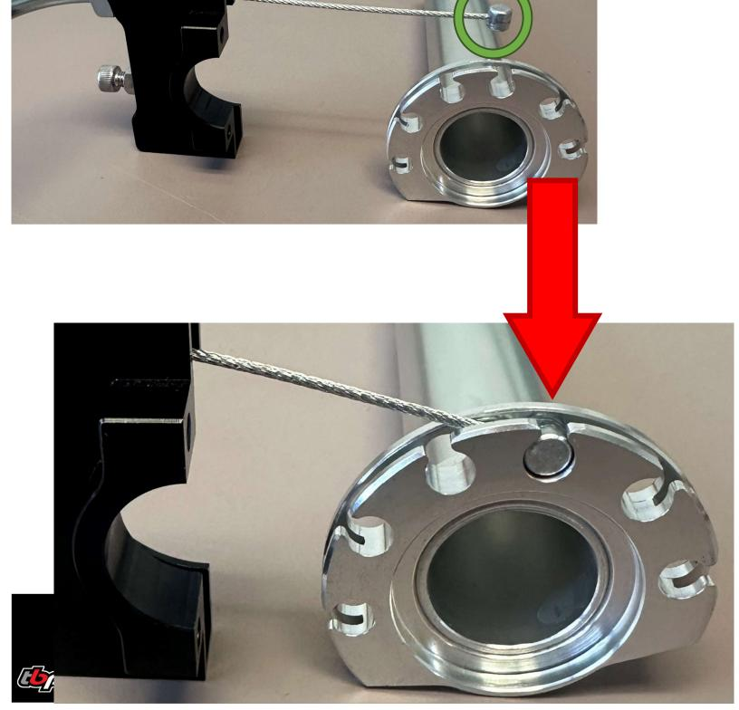
Rest the flat part of the throttle on top of the safety stop bolt.
