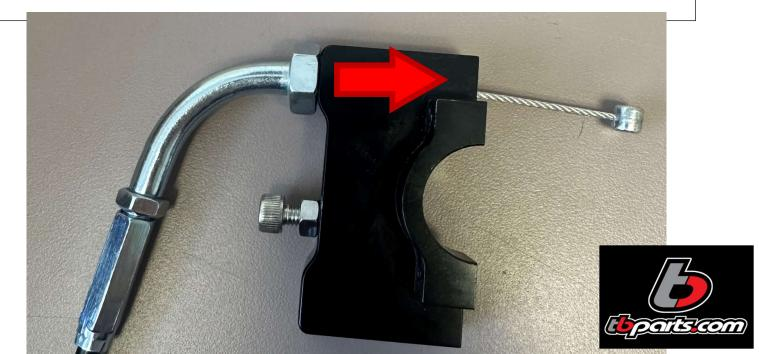
Attach the barrel end of the cable to the throttle tube.
