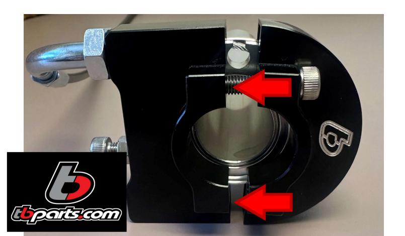
Insert bolts and tighten.
