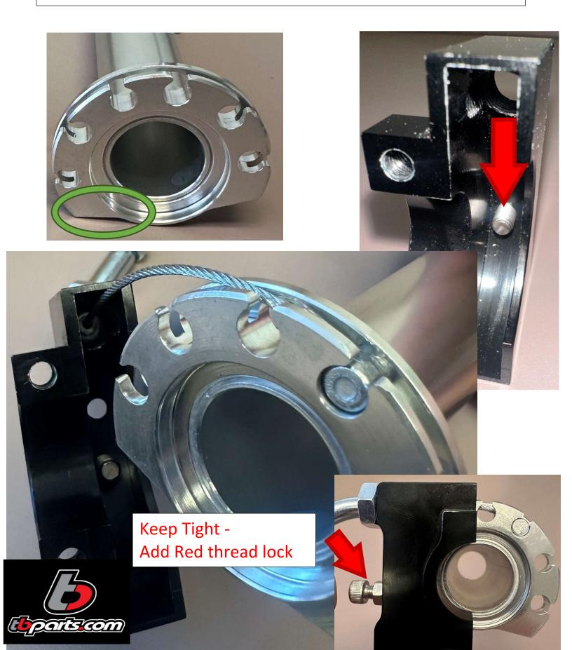
Once in place, align cover billet piece with corresponding bolt holes.
